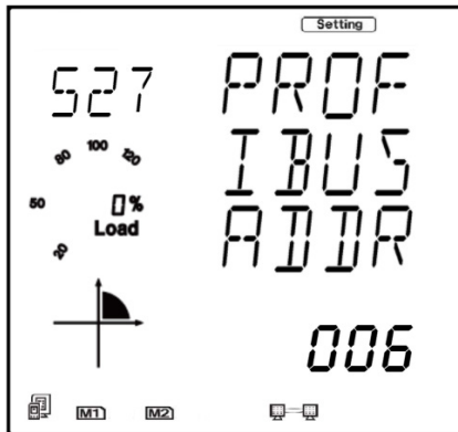
Figure 5-50 AXM-PROFI address setting on meter display
