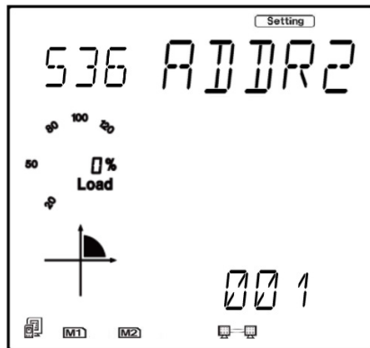
Figure 5-55 Address setting for AXM-RS485
