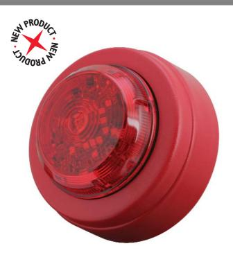
The Solista MAXI is an enhancement of the standard Solista LED beacon which allows the user the choice between economy or performance. In the economy modes the Solista MAXI performs extremely efficiently requiring as little as 3mA, but it can be switched to attain much higher light outputs where visibility is the prime objective. For even greater effectiveness a double flash sequence can be selected.
