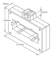
• Hole for M6 diameter screws or busbar mounting
