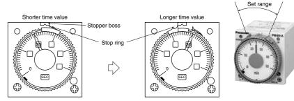
Note) The stoppers for the lower limit setting set ring and the upper limit setting set ring face the opposite directions.
