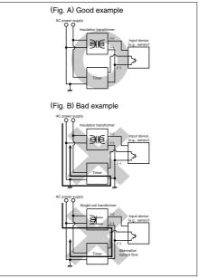
Do not use a single coil transformer (e.g., Sly-Duck). Otherwise, the internal circuit of the timer will be short-circuited as shown in Fig. B resulting in breakdown
