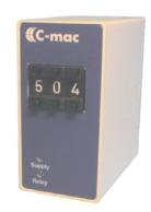
C-mac<sup>®</sup> module type RD53 is a digital pulse counter module, selectable as pulse divider or preselection relay. The pulse inputs can be activated from a mechanical contact, a transistor or a NAMUR sensor, and the reset input can be activated from a mechanical contact or a transistor. The unit is supplied with a "slave" transistor output, in this way several units can be connected to the same pulse sensor.
