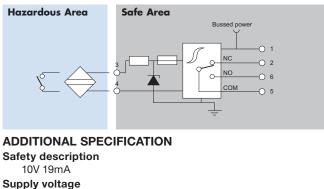
22.9 to 30V dc with respect to earth Input characteristics Relay energised if input >2.1mA(<2k $\Omega$ )
