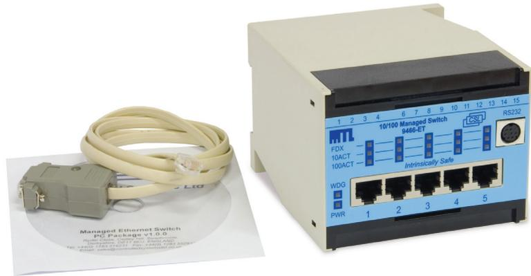
The 9466-ET 10/100Mbps, Layer 2, Ethernet switch allows the interconnection of MTL 9400-ET series networking modules via its 5 ports. It also enables an Ethernet network to cover a greater distance using either Cat5e cable or fibre-optic for longer spans. This capability is due to the low latency 'store and forward' mechanism integral to the switch, which ensures that the stringent timing associated with Ethernet is maintained.
