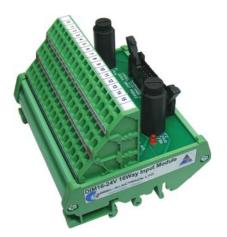
The DIM16-24V digital input module has a three tier spring clamp terminal block. The top row has the 16 active high inputs (A0 to A15) plus two fuse blown (FB) active high output terminals. The middle row has two fused groups of eight 24V supply outputs plus two 24V supply input terminals. And the bottom row has 18 0V supply terminals.
