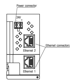
Fig. 4.1 Device's connectors
