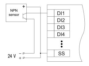
Fig. 4.7 Connection of NPN transistors (only for MV210-202)
