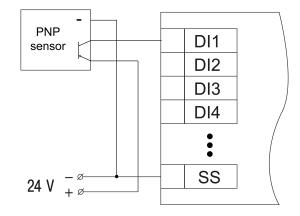
Fig. 4.6 Connection of PNP transistors (only for MV210-202)
