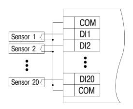
Fig. 4.4 Connection to the inputs DI1-DI20 (MV210-202)
