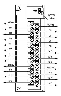
Fig. 4.3 Terminal block layout
