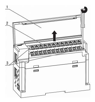
Fig. 7.1 Remove terminal block
