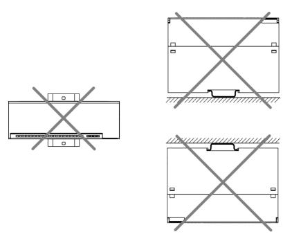
Fig. 3.2 Improper installation
