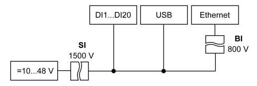
Fig. 2.1 Isolation of the Device Components
