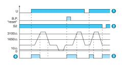
The relay is reset either using the RESET pushbutton on the front face or by opening the external contact \$2 (remote reset), or by cutting the auxiliary power supply (terminals A1 - A2). If the auxiliary power is cut for a period of time greater than the reset time (500 ms), the relay is reactivated if the proble detects a normal temperature when the power supply voltage is restored.
