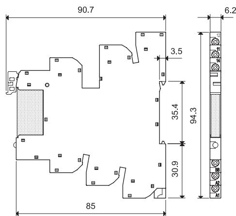
**Electromechanical Relay (1 Pole 6 A) & Socket Combinations**
