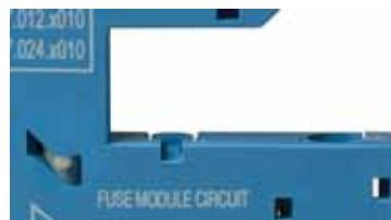
3. In order to reinstate the output circuit it is necessary to either re-insert the fuse module (complete with functional fuse), or alternatively, return the peg/indicator to position 0 by gently applying pressure in the direction of the arrow.
