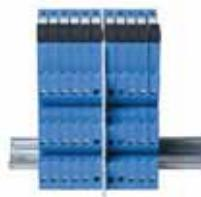
2. Leaving the ribs in place provides 6.2mm separation. Simply cutting (with scissors) the relevant segment(s) permits the interconnection across the separator of 2 different groups of interface relays, using the standard jumper link.
