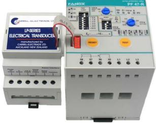
The Fanox pump protection relay interface is designed to provide isolated status outputs for remote monitoring of the PF series relays. The unit plugs into the accessory socket on the top of the PF series relays.
