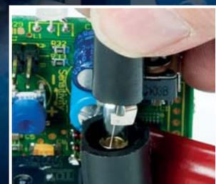
MP15P internal replaceable fuse
