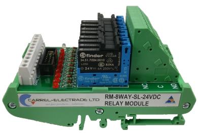
The relay module provides 8 relays, either the electromechanical Finder 34.51 24VDC relays, or the solid-state Finder 34.81 24VDC relays. The relay module can be populated with a mixture of electromechanical and solid-state relays to suit the loads being switched. The module is suitable for low-voltage use only - voltages up to 36V.
