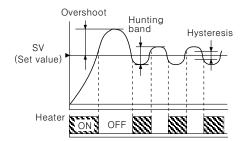
As like above picture, the control value is up and down by set value, it is called Hunting. And Overshoot is occurred at initial point when just power on
