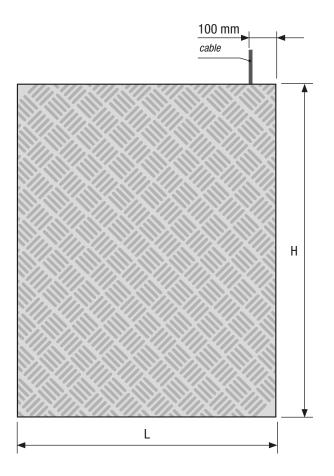
*The safety mat is equipped with a 4-pole, FROR 300/500, outlet cable (4x0.35mm2) – standard length 3 m - placed at a distance of 100 mm from the right edge.*
