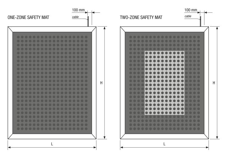
The safety mat is equipped with a 4-pole, FROR 300/500, outlet cable (4x0.35mm2) – standard length 3 m - placed at a distance of 100 mm from the right edge.
