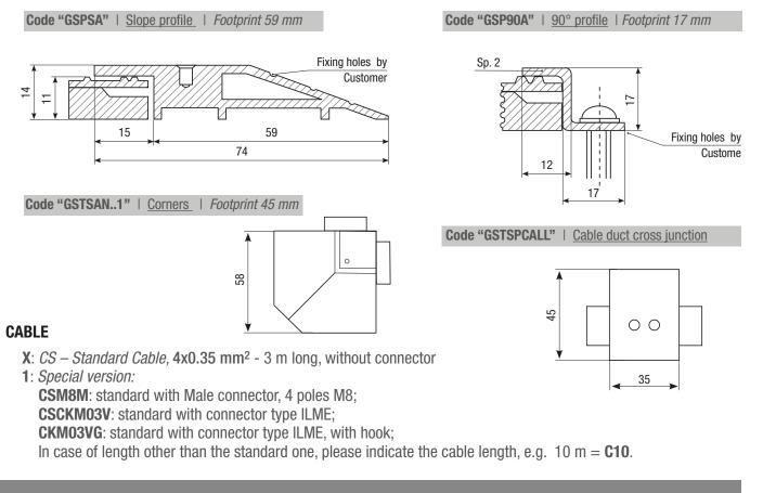
*Example:* safety mats with mounted profiles, dimensions 1000x1000, with slope profile on 4 sides and with standard cable outlet.
