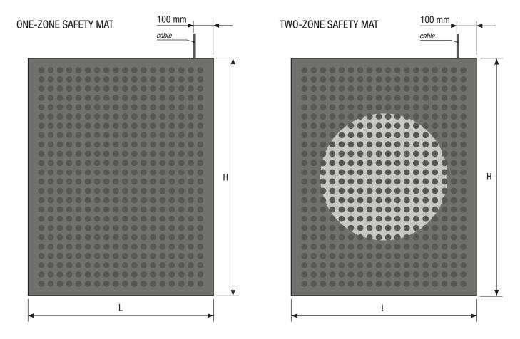
The safety mat is equipped with a 4-pole, FROR 300/500, outlet cable (4x0.35mm2) – standard length 3 m - placed at a distance of 100 mm from the right edge.
