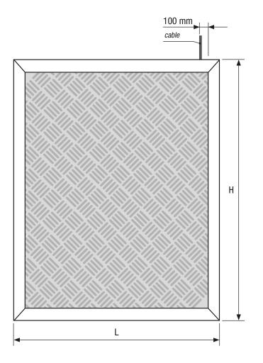
*The safety mat is equipped with a 4-pole, FROR 300/500, outlet cable (4x0.35mm2) – standard length 3 m - placed at a distance of 100 mm from the right edge.*
