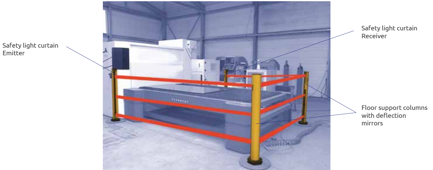
Fig. 26. Machine for laser cutting perimeter protection
