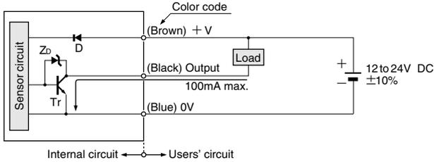
Symbols ... D: Reverse supply polarity protection diode
