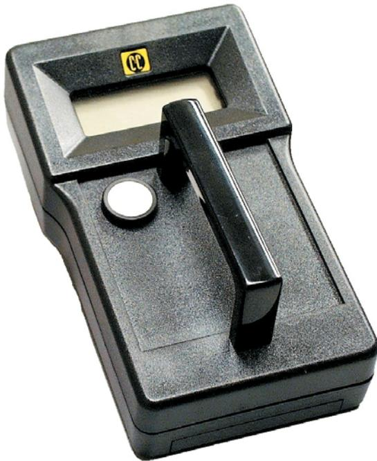
The C301 capacitive timber moisture meter is non-invasive and simple to use. No large electrodes or pins are required to be inserted into the timber.
