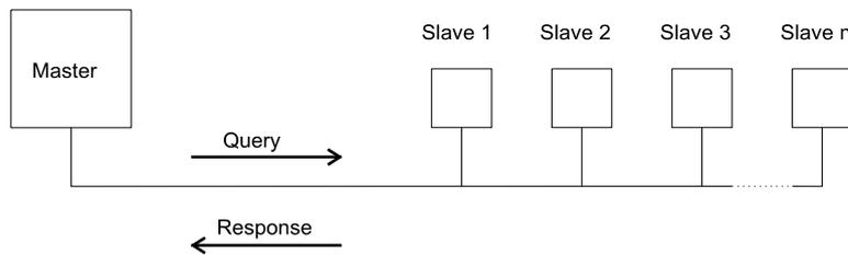
In the MODBUS Protocol the master can address individual slaves, or, using a special “Broadcast” address, can initiate a broadcast message to all slaves. The Dual Load Digital meter does not support the broadcast address.
