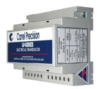
The LP-1V3 three phase var transducer converts ac current and voltage signals into a load independent bidirectional dc signal proportional to the reactive power flowing in the system. The transducer is designed for 3 phase 3 wire systems with a balanced supply and a balanced load.
