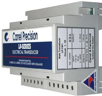
The LP-1W1 single phase Watt transducer converts ac current and voltage signals into a load independent bidirectional dc signal proportional to the active power flowing in the system.
