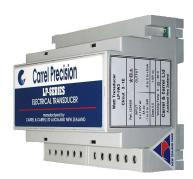
The LP-1W3 three phase Watt transducer converts ac current and voltage signals into a load independent bidirectional dc signal proportional to the active power flowing in the system. The transducer is designed for 3 phase 3 wire systems with a balanced supply and a balanced load.
