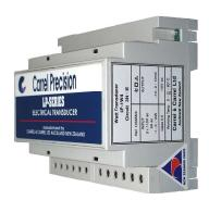
The LP-1W4 three phase Watt transducer converts ac current and voltage signals into a load independent bidirectional dc signal proportional to the active power flowing in the system. The transducer is designed for 3 phase 4 wire systems with a balanced supply and a balanced load.
