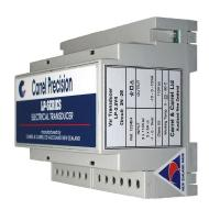
The LP-2.5V4 three phase var transducer converts ac current and voltage signals into a load independent bidirectional dc signal proportional to the reactive power flowing in the system. The transducer is designed for 3 phase 4 wire systems with a balanced supply and an unbalanced load.
