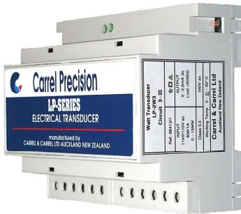
The LP-2.5W4 three phase Watt transducer converts ac current and voltage signals into a load independent bidirectional dc signal proportional to the active power flowing in the system. The transducer is designed for 3 phase 4 wire systems with a balanced supply and an unbalanced load.
