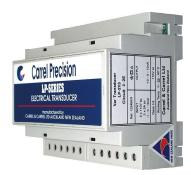
The LP-2V3 three phase var transducer converts ac current and voltage signals into a load independent bidirectional dc signal proportional to the reactive power flowing in the system. The transducer is designed for 3 phase 3 wire systems with a balanced supply and an unbalanced load.
