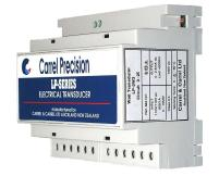
The LP-2W3 three phase Watt transducer converts ac current and voltage signals into a load independent bidirectional dc signal proportional to the active power flowing in the system. The transducer is designed for 3 phase 3 wire systems with a balanced supply and an unbalanced load.
