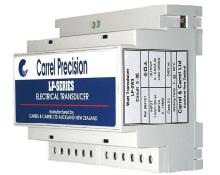
The LP-3W4 three phase Watt transducer converts ac current and voltage signals into a load independent bidirectional dc signal proportional to the active power flowing in the system. The transducer is designed for 3 phase 4 wire systems with an unbalanced supply and an unbalanced load.
