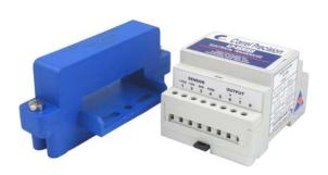
The LP-CDU-BP-HALL is a special version of the LP-CDU transducer which converts the signal from a Hall effect sensor (DC current transformer) into a standard transducer output. It also supplies the ±15Vdc power supply for the Hall effect device.
