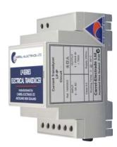
The LP-IP and LP-IL current transducers convert an ac current input into an output signal which is proportional to the rms calibrated rectified arithmetic mean of the input.
