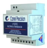
The LP-TPR resistance type tap-position transducer converts a potentiometric voltage into a load independent dc current or voltage signal.
