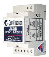
The LP-TR temperature transducer converts the resistance value of a platinum resistance element into a load independent dc current or voltage signal. The three wire method of measurement employed ensures that balanced cable resistance values can be accommodated without affecting the accuracy of the reading. The circuitry employed corrects the non-linear response of the Pt100 to yield a signal proportional to temperature.
