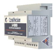
The LP-VPW window transducer and LP-VP-DSW dual slope transducer convert ac voltage inputs into an output signal which is proportional to the rms calibrated rectified arithmetic mean of the input.
