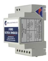
The LP-VP and LP-VL voltage transducers convert an ac voltage input into an output signal which is proportional to the rms calibrated rectified arithmetic mean of the input.
