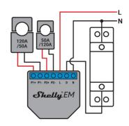
SHELLY-EM-50A WI-FI ENERGY METER 50A 110-230VAC WITH 50AMP CLAMP CT
