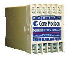
The Carrel Electrade T-IS current transducer converts a sinusoidal ac current into a load independent dc current or voltage signal capable of driving a number of independent instruments. Power for this unit is derived from the input signal. The output signal is calibrated to rms, based on an arithmetic mean measurement of the rectified input signal, and hence the transducer should be used with undistorted sine waveforms (<1% distortion).
