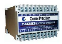
The T-TPA ac reluctance type tap-position transducer converts ac voltages derived from an excited variable reluctance tap-position source into a load independent dc current or voltage signal capable of driving a number of independent instruments. The transducer measures both the excitation and output voltage from the tap-position source and generates an output that is proportional to the quotient of these two signals.
