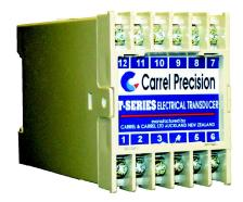
The Carrel Electrade T-TPR resistance type tap-position transducer converts a potentiometric voltage into a load independent dc current or voltage signal capable of driving a number of independent instruments. Power for the unit is derived from an auxiliary supply.
