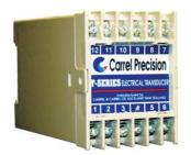
The T-VP voltage transducer converts a sinusoidal ac voltage input into a load independent dc current or voltage output. Power for the unit is derived from an auxiliary supply. The output is proportional to the rms calibrated rectified arithmetic mean of the input. Accurate measurement assumes a sinusoidal input waveform. The auxiliary power supply allows low input burdens, high sensitivity and live zero outputs, eg 4-20mA.
