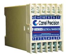
The Carrel Electrade T-VS voltage transducer converts a sinusoidal ac voltage into a load independent dc current or voltage signal capable of driving a number of independent instruments. Power for this unit is derived from the input signal. The output signal is calibrated to rms, based on an arithmetic mean measurement of the rectified input signal, and hence the transducer should be used with undistorted sine waveforms (<1% distortion).
